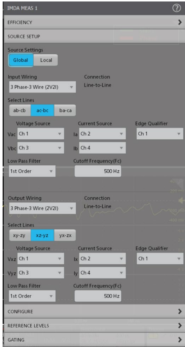
Figure 32. Setup for configuring a 3-wire input and 3-wire output for efficiency measurements using a 5/6 Series MSO oscilloscope.
