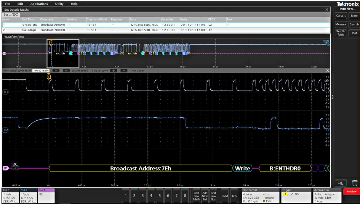
The Protocol Decode Results Table provides a time-stamped, tabular view of all captured packets on the I3C bus.
