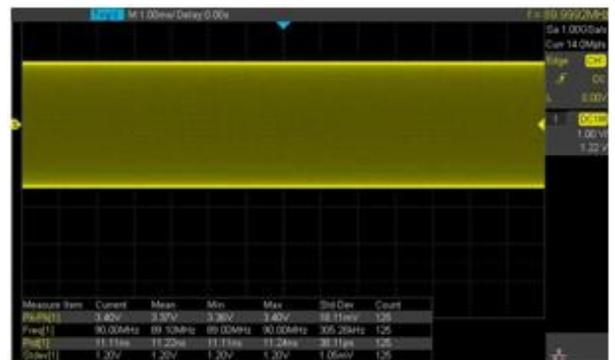
At any one timebase, ADS-4000 can measure using all 14M sample points. This ensures the accuracy of measurements while the math co-processor decreases measurement time and increases ease-of-use.
