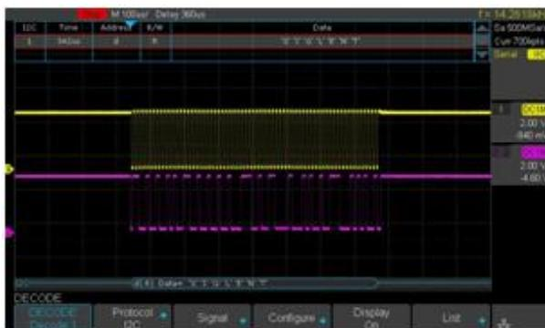
ADS-4000 displays the decoding through the events list. Bus protocol information can be quickly and intuitively displayed in table form.
