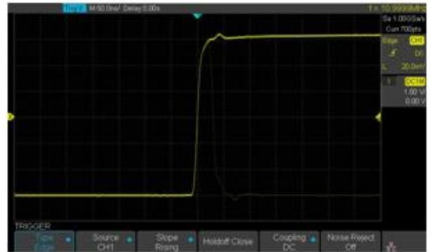
With a waveform capture rate of up to 400,000 wfms/s (sequence mode), the oscilloscope can easily capture the unusual or low-probability events.
