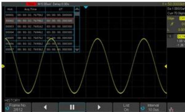
Playback the latest triggered events using the history function. Segmented memory collection will store the waveform into multiple (Up to 80,000) memory segments, each segment will store triggered waveforms and timestamp each frame.
