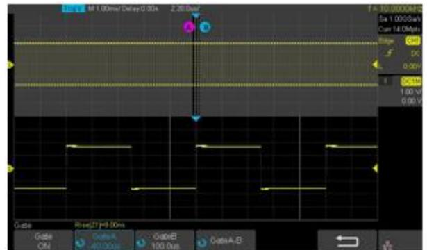
Through Gate and Zoom measurement, you can specify arbitrary waveform interval of data analysis and statistics to avoid measurement errors caused by invalid data.
