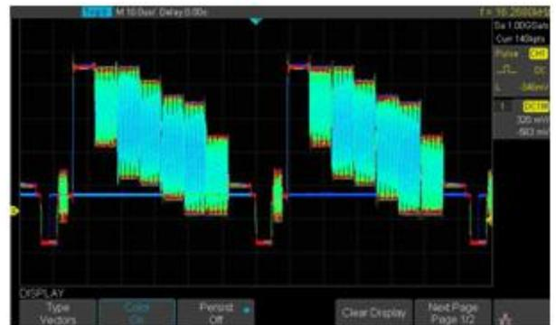
The color temperature display is similar to the intensity-graded trace in function, except that the trace occurrence is represented by different colors (color "temperature") as opposed to changes in the intensity of one color. Red represents the most common occurrences or probabilities, while blue is used to mark points that occur least frequently.
