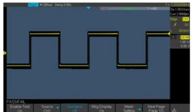
The ADS-4000 utilizes a hardware-based Pass/Fail function, performing up to 40,000 Pass / Fail decisions each second. Easily generate user-defined test templates provide trace mask comparison making it suitable for long-term signal monitoring or automated production line testing.
