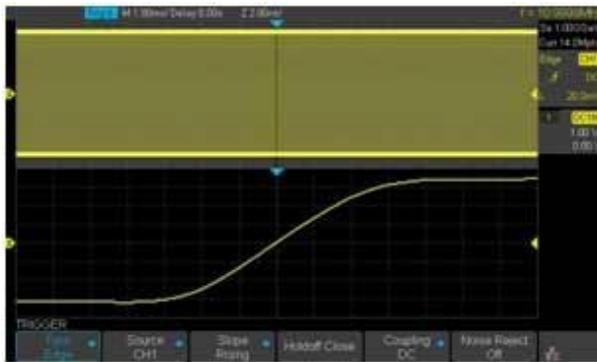
Using hardware-based Zoom technologies and a record length of up to 14 Mpts, users are able to use a higher sampling rate to capture more of the signal and then quickly zoom in to focus on the area of interest.
