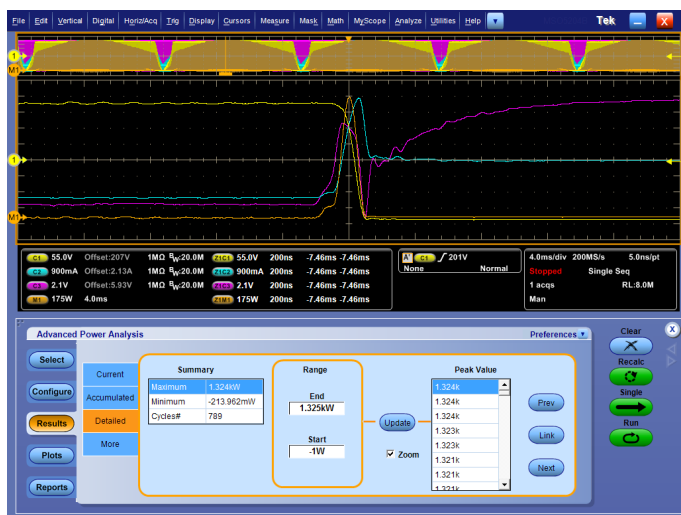
FIGURE 13. HiPower Finder identifying peak losses in MOSFET switching loss measurements.
