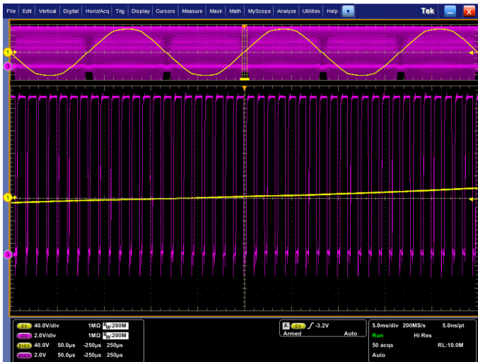
FIGURE 8. The AC input voltage and the modulated Gate voltage on the switching MOSFET.
