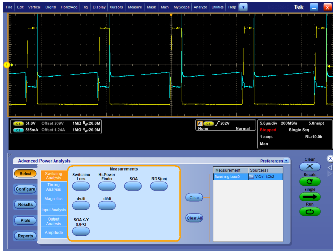
FIGURE 10. PFC voltage and current measurements.
