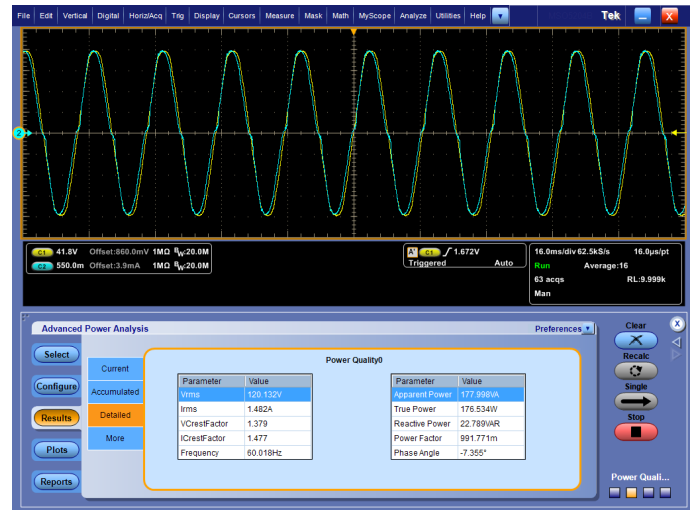
FIGURE 4. Power Quality measurements on PFC give power factor readings in addition to true power, apparent power, reactive power, and phase angle.
