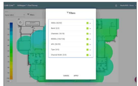
Filters allow you to choose the types of devices and network configurations to be shown.
