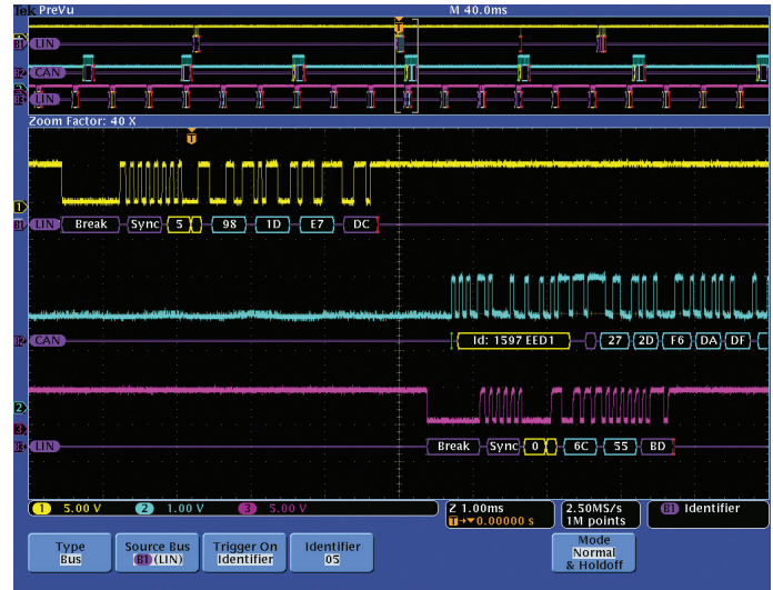
Figure 36. Simultaneous capture and decode of multiple automotive serial buses.
