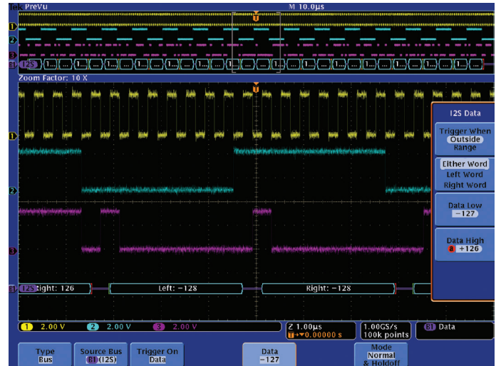
Figure 49. Triggering outside a range of values on an I 2 S bus.
