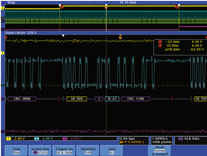
Figure 31. Triggering on specific identifier and Data on a CAN bus and decoding all messages in the acquisition.
