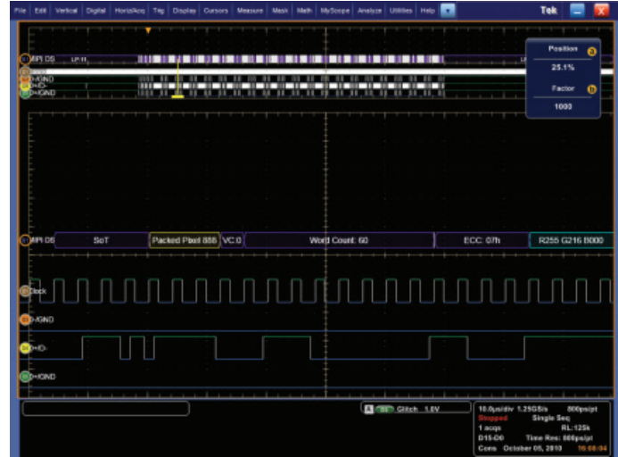
Figure 53. MSO70000C digital-channel decoded display of a Packed Pixel Stream, 24-bit RGB 8-8-8 Format long packet.
