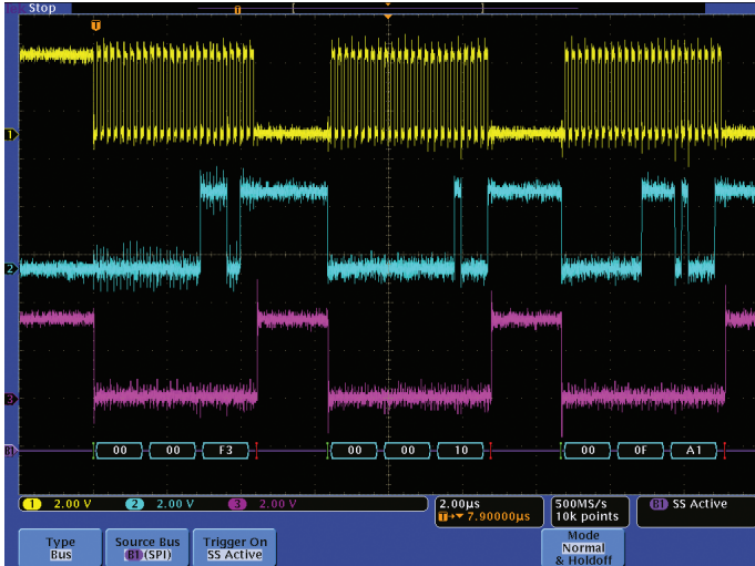
Figure 13. Correct synthesizer configuration messages.
