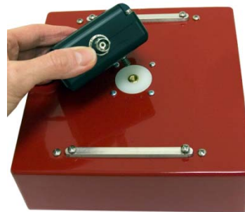
Insert mounting stud into rod element mounting hole and rotate to tighten
