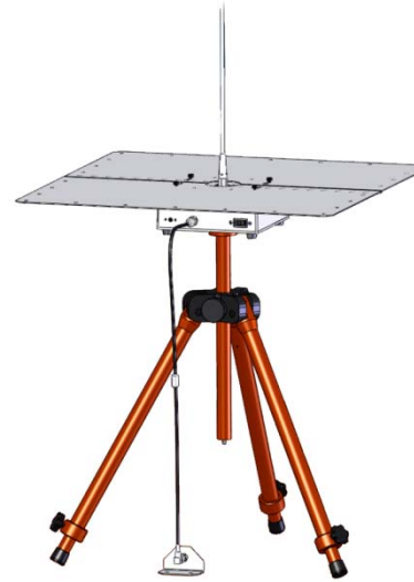
Model 3301C shown mounted with MIL-STD-461F Test Kit onto 4-TR Light Tripod
