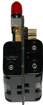
Vertical board with four batteries
