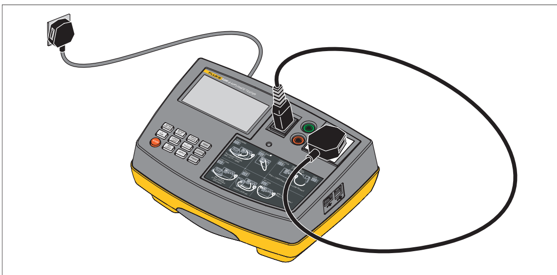
Figure 6. IEC-Lead Test Connections
