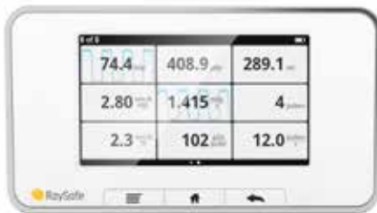
HOME SCREEN Measurement of 1 – 12 parameters simultaneously with waveform overlay.
