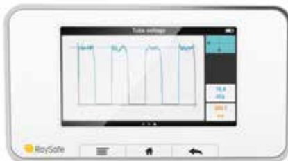
WAVEFORM Overview and simple analysis of kVp, dose rate or mA.
