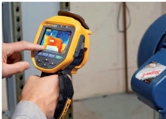
Fluke Ti480 Pro used for motor inspections
