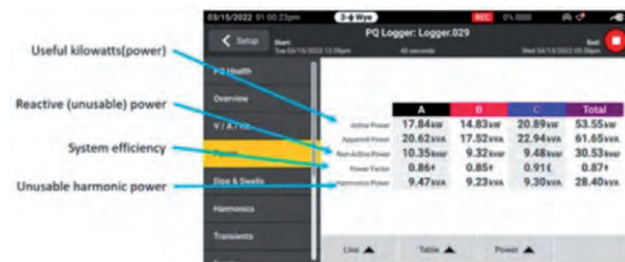
Image 4: Useful and unusable power captured by the Fluke 1777
