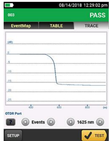
Splitter as seen on an OTDR trace
