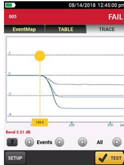
Bend as seen on an OTDR trace
