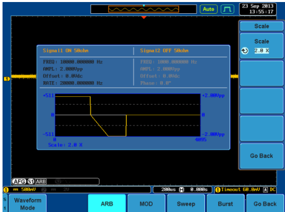
Figure of 2.0X scaling. Notice that the waveform is clipped at the bottom.
