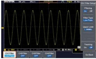
Filtered Waveform, Noise Removed
