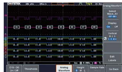
Display analog waveform converted from digital signal
