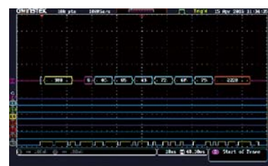
CAN Bus Trigger and Decode
