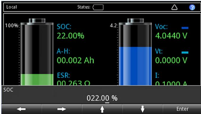
**Figure 4.** Initiate battery condition in battery simulation mode.
