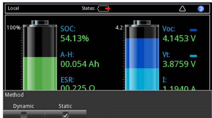
**Figure 6.** Dynamic and static modes in battery simulation.
