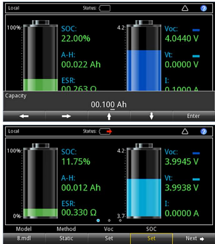
**Figure 5.** Modify battery capacity to accelerate charge/discharge tests.
