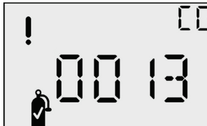
Cal Failed (!) Screen
