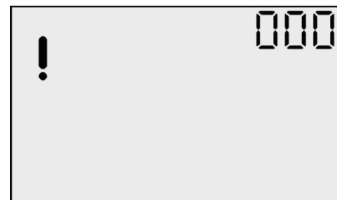
Sensor Missing Error Screen
