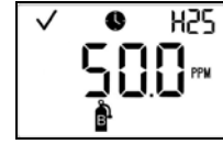
Bump test apply gas
