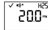
High alarm setpoint
