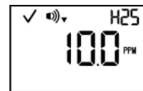
Low alarm setpoint
