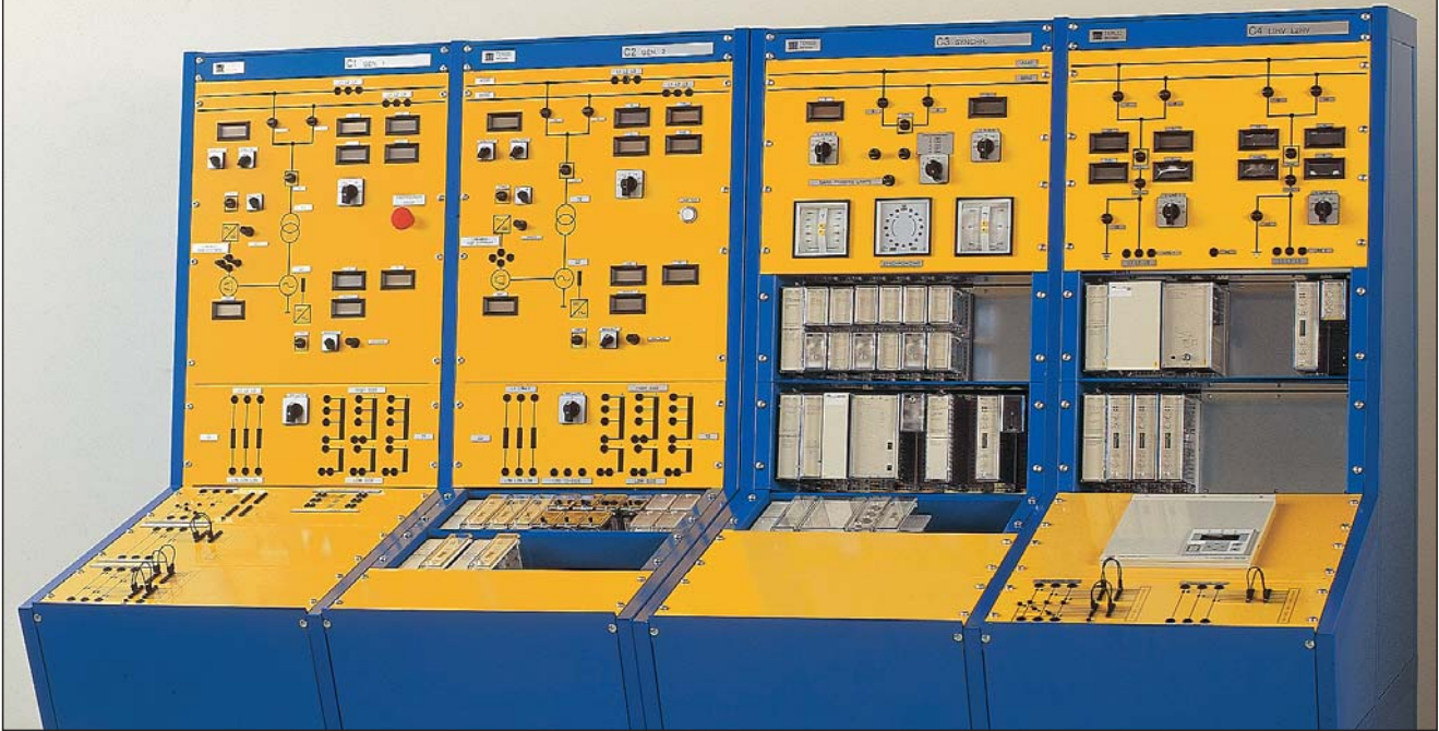
PST 2210, The Power Plant Simulator above is an extended version with two turbine-generator sections, fully equipped with all protective relays and step-up transformers. The standard version has one fully equipped turbine-generator section.
