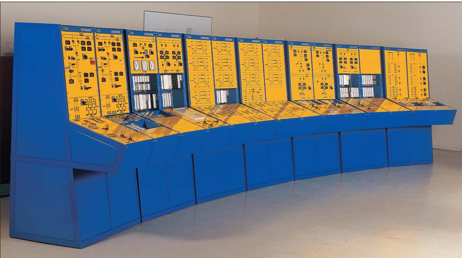
Different set ups of the Power System Simulator. Due the modular system, the system can be arranged in different ways depending on the available space.
