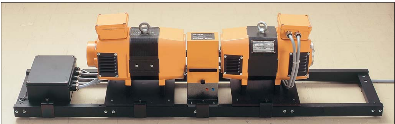
Turbine Generator Set: The power is generated by a 3-ph synchronous generator driven by a separately excited DC-motor as turbine. The electrical machines set is electrically fully connected and mechanically mounted on a machine bed.
