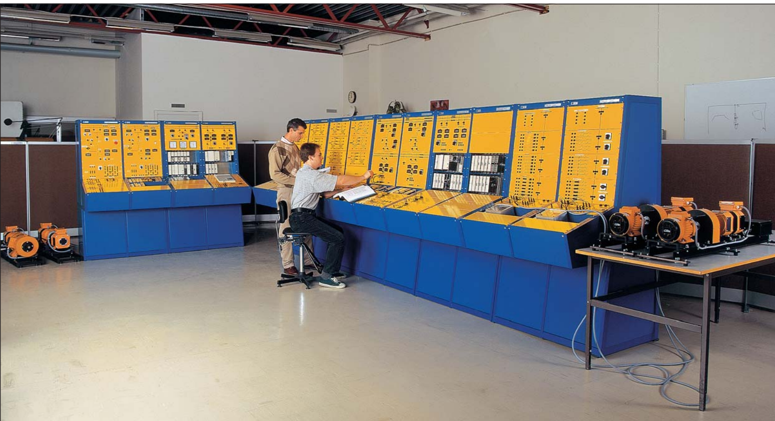
Different set ups of the Power System Simulator. Due the modular system, the system can be arranged in different ways depending on the available space.
