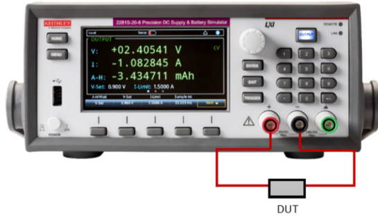
Two-wire (local sensing) DUT connection to front panel
