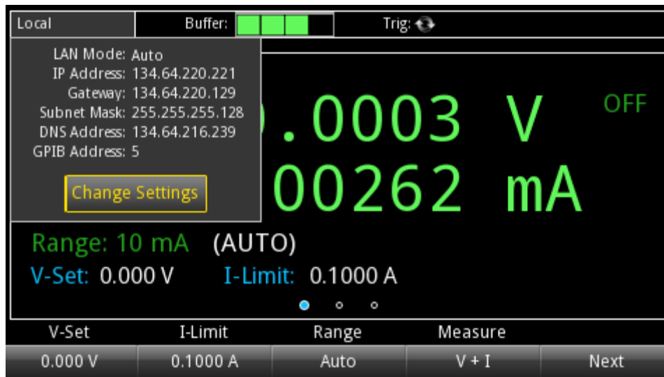
Figure 5: 2281S-20-6 communication status indicator
