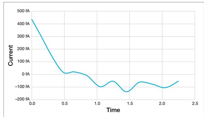
The S535 quickly settles a to sub-200 fA noise floor (12 V @ 1 PLC measurement speed).
