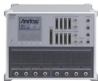
MD8430A Signalling Tester
