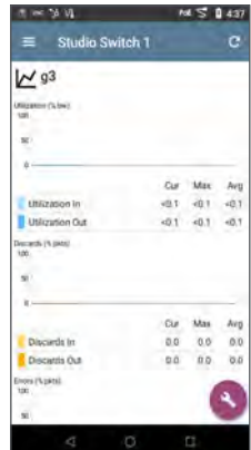
Interface traffic statistics - correlated for 24 hours to detect intermittent events
