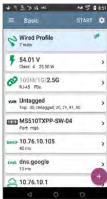
NBASE-T network with VLAN and 802.1x authentication
