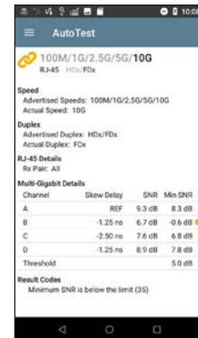
Cabling SNR measurement validates Multi-Gig links
