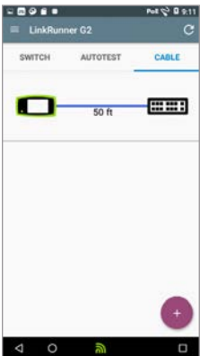
Distance to Open while connected to Switch
