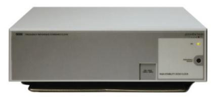
The Pendulum Frequency References; model 6689 with a Rubidium clock and model 6688 with a high-stability oven-controlled crystal oscillator, are designed for use in test systems, where a very high stability frequency reference is required and where multiple instruments or testers need to be supplied.
