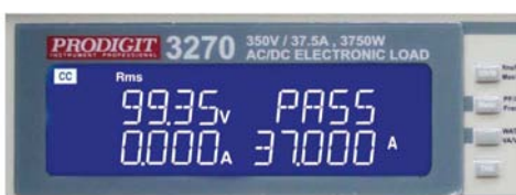
Turbo OFF, Short 100ms 37.5A Test result screen
