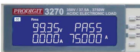
Turbo OFF, Short 100ms 37.5A Test result screen
