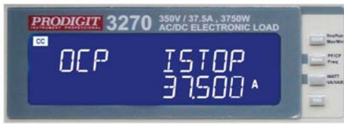
Turbo OFF, OCP Istep 3.75 A Istop 37.5A Test result screen
