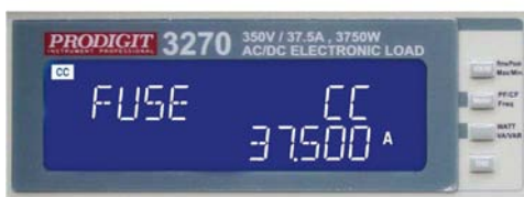
Turbo : OFF, Fuse mode Test result screen
