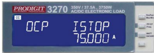
Turbo ON, OCP Istep 7.5 A Istop 75A Test result screen
