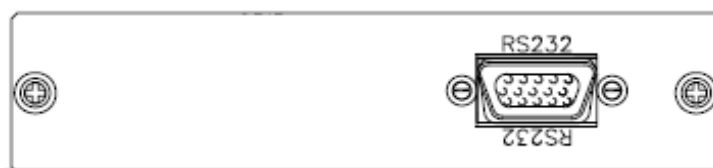
Fig 2-3 36000A Series RS232 Rear panel
