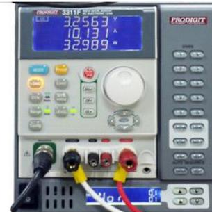
3311F Electronic load on 3302 mainframe
