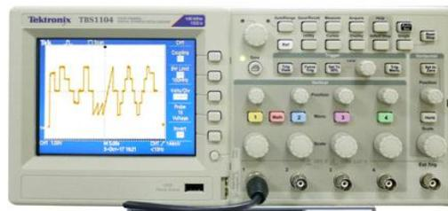
Actual load current waveform on DSO
