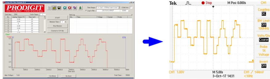
Edit by 9923 application software    Regeneration the load current waveform
