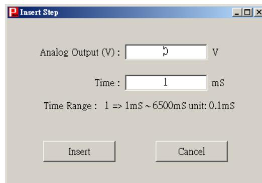
1. Analog Output (V) : Set the analog output voltage.
