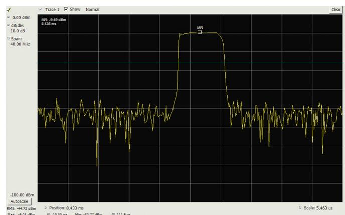
Figure 14. Amplitude vs. time with no trace decimation.
