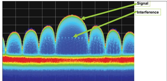
Figure 31. The RSA with DPX Live RF spectrum display can see the interfering signal hopping underneath the radar pulse.
