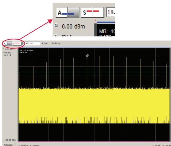
Figure 13. Time overview of the Weather Radar.
