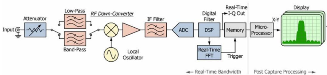
Figure 7. Alternate instrumentation block diagrams.
