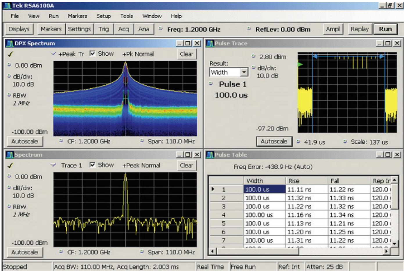
Figure 25. RSA measurements of the Frank Coded pulse.
