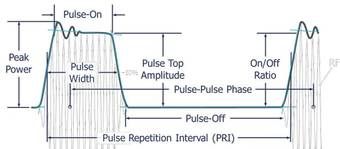
Figure 1. The autonomy of a pulse.
