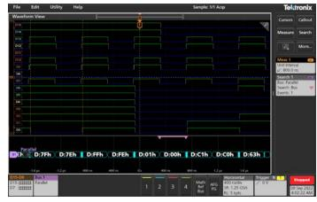
Digital channel trigger and decode
