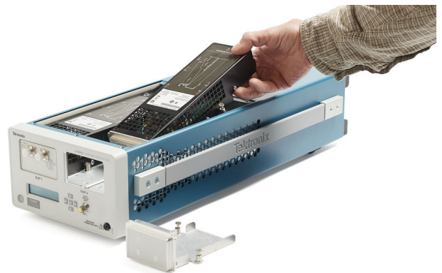
Figure 2: Plugging TSO8C18 module into TSO820 mainframe.
