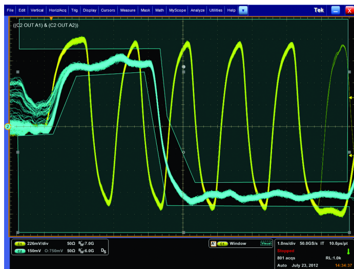
DDR memory. Visual Trigger used to isolate a rare occurrence of a write burst on a specific bit pattern in DDR3. The trigger event is a Write DQ burst of 11000000, when the DQ launch starts from a non-tri-state voltage value. DDR memory bus events involve clocks, strobes and data channels as well as multiple amplitudes and bursts of data.
