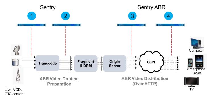
For OTT, TV Everywhere and Multiscreen video service monitoring, customers typically use the Sentry Video Quality Monitor at the ABR video content preparation stage (pre- and post-transcode) for in-depth QoE (Quality of Experience) monitoring and analysis. Sentry ABR is used at the ABR Video Distribution stage for QoS (Quality of Service) monitoring of all ABR files and fragments.
