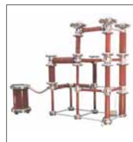
3-stage DC Voltage Test Set-up
