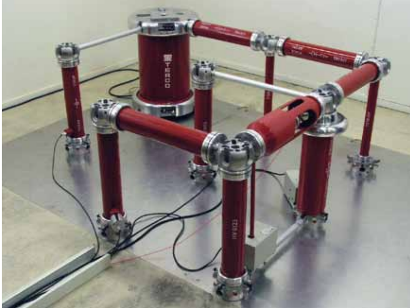
Single stage Impulse Voltage Test Set-up (In the picture above AC-divider + Connecting Rod incl.)
