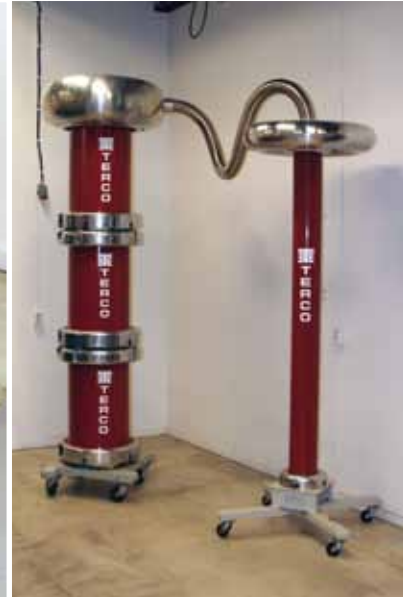
3-stage AC Voltage Test Set-up
