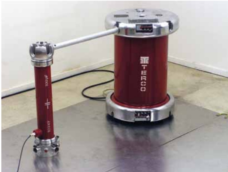
Single-stage AC Voltage Test Set-up
