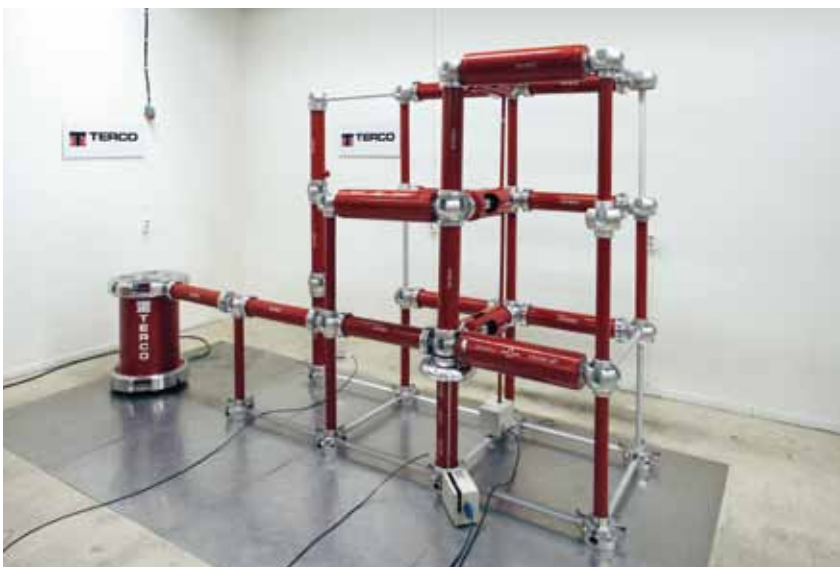
3-stage Impulse Voltage Test Set-up
