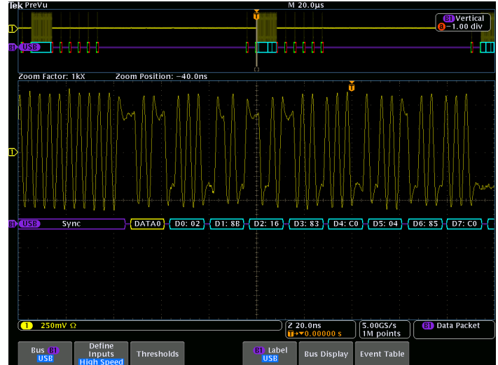
High-speed USB decoded display, automatically displaying bus content in any of several digital formats
