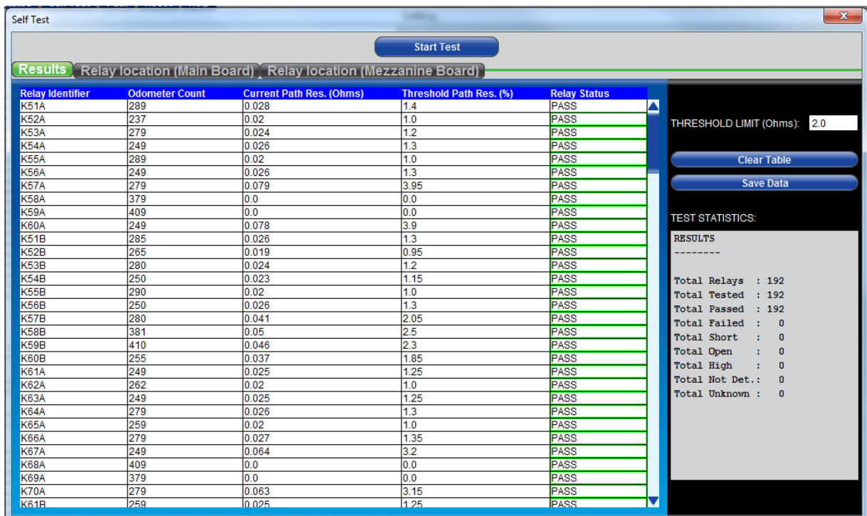
FIGURE 3-13: SELF TEST GUI – POST SELF TEST COMPLETION, SCREEN SHOWING THE TEST STATISTICS
