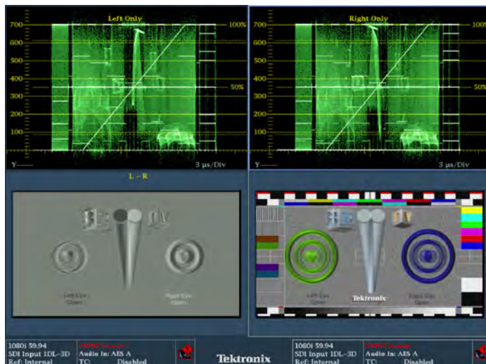
Simultaneous 3D display of Left Eye and Right Eye signals with Difference Map and Overlay picture displays.
