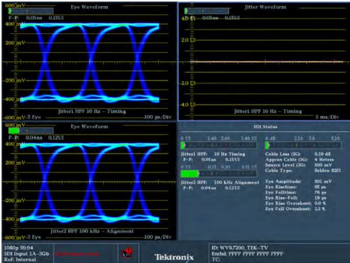
Eye and Jitter display along with automated measurements of physical layer parameters.
