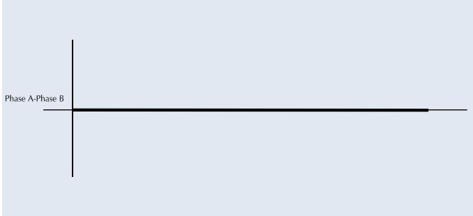
Figure 4. Identical pulse waveform on all three phases results in zero voltage.
