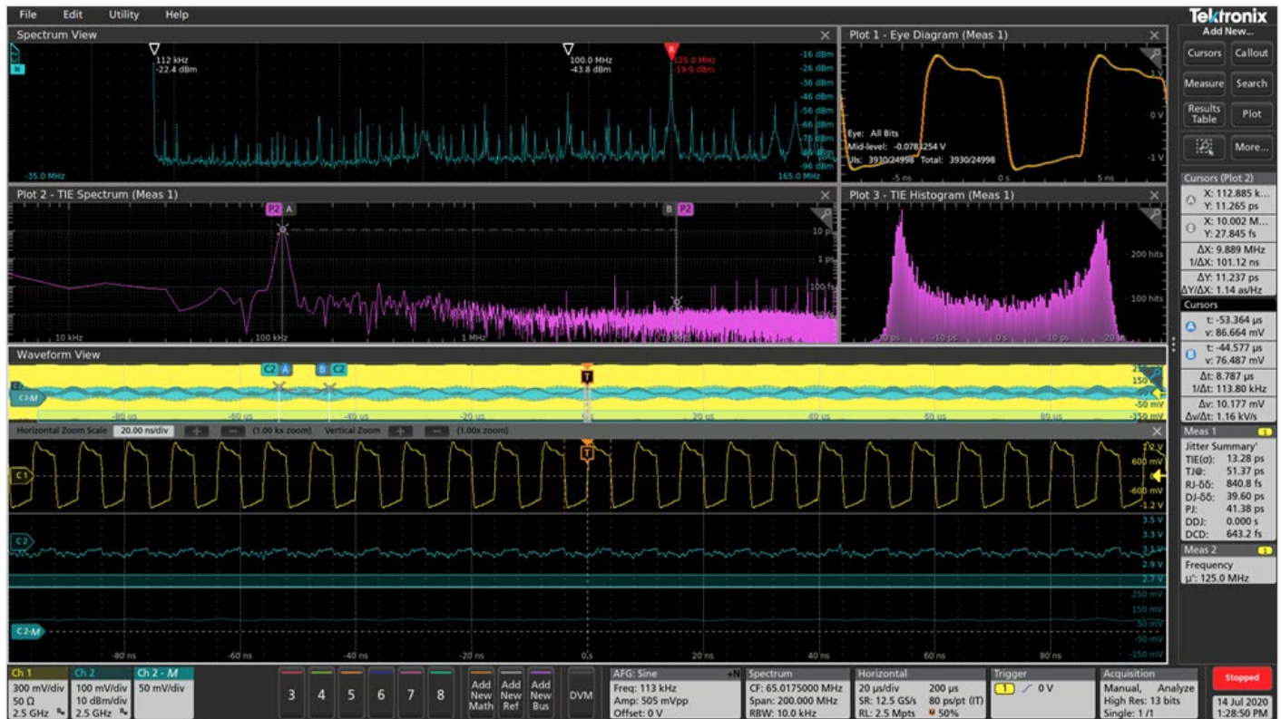
Figure 8: (a) Power rail ripple spectrum and (b) TIE/ jitter spectrum.
