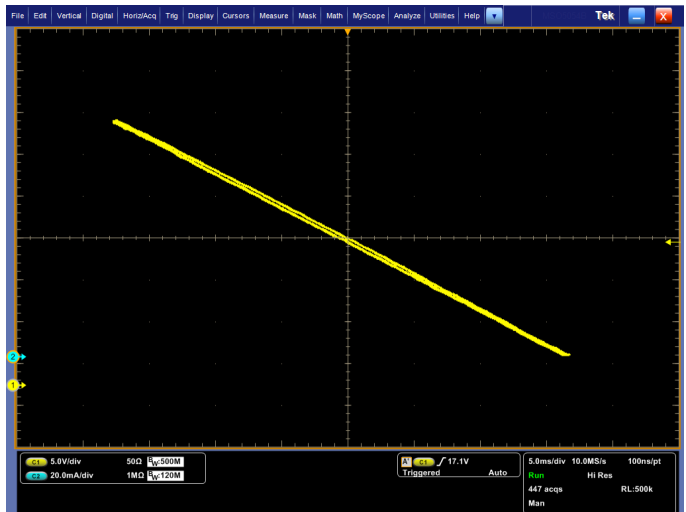
FIGURE 7. Linear X-Y oscilloscope display of switch voltage and current.
