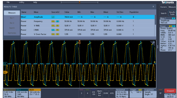
Figure 11. Power Quality Measurements.
