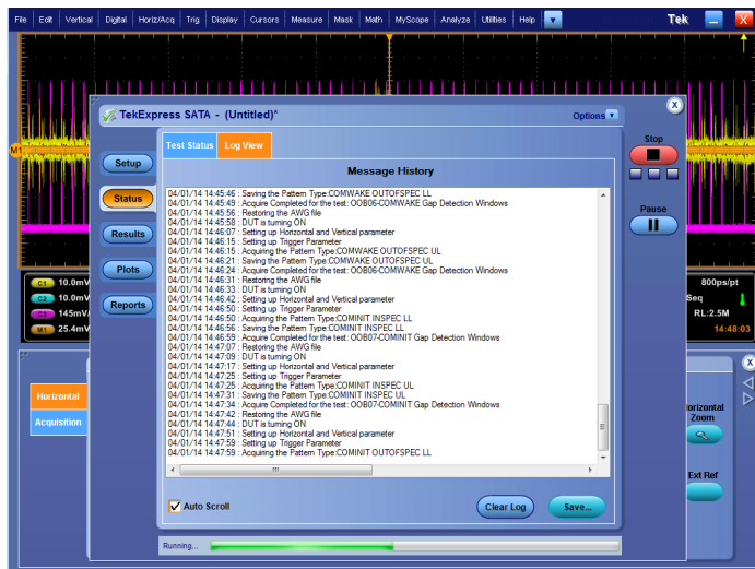
Step-by-step status view of BIST-L negotiation, pattern validation, signal acquisition and analysis
