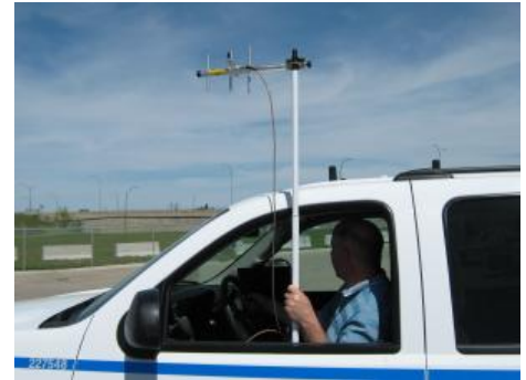
"Broom stick" antenna used for directional interference chasing and hooked up to the Tektronix RSA306B spectrum analyzer.
